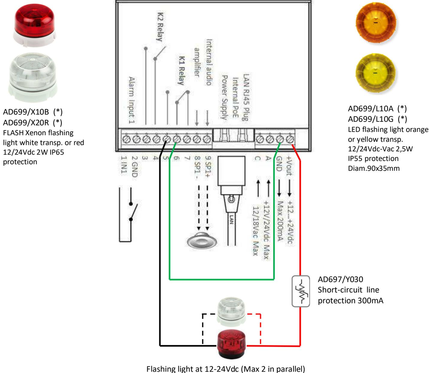
Connect the flash light to the terminal + Vout with the red wire (possibly interposing a short-circuit protection), connect the black flash light wire to terminal number 5 of the module, then make a bridge with wire between terminal number 6 and terminal called GND. Then program in the "Relay and alarm inputs settings" screen the relay 1 in "2 - In Call" mode and press "APPLY" (see next page), in this way the flash light will be activated for the duration of the announcement or communication.
